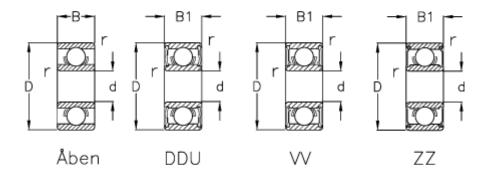
Max rpm ZZ-WW = 34000 В = 7 B1 = 7 r min = 0.3Type = 608 d = 8 D = 22 Load Cor (N) = 1370Load Cr (N) = 3300 Max rpm DD = 28000
